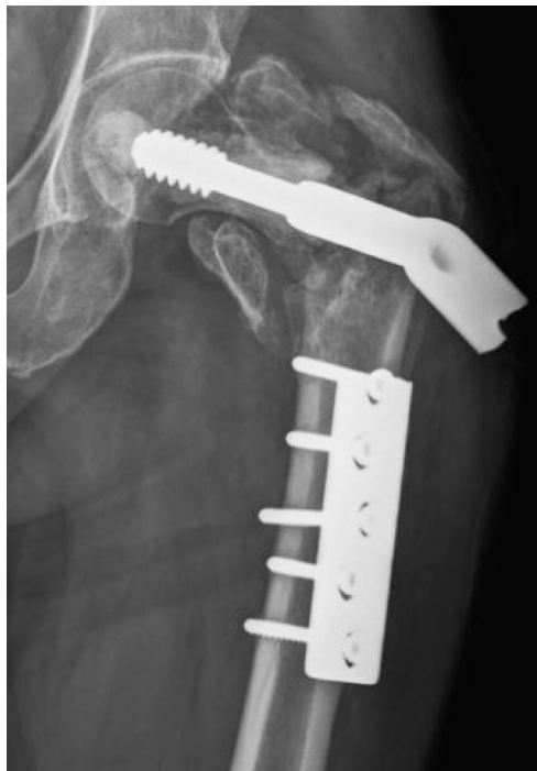
Fig. 2 Side plate breakage from the screw hole.
