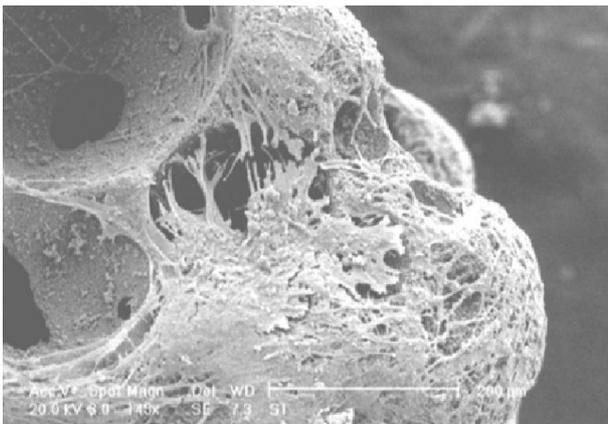
**Fig. 5** Relatively normal distribution of MSCs on the HA/TCP scaffolds (high magnification 1/100)
